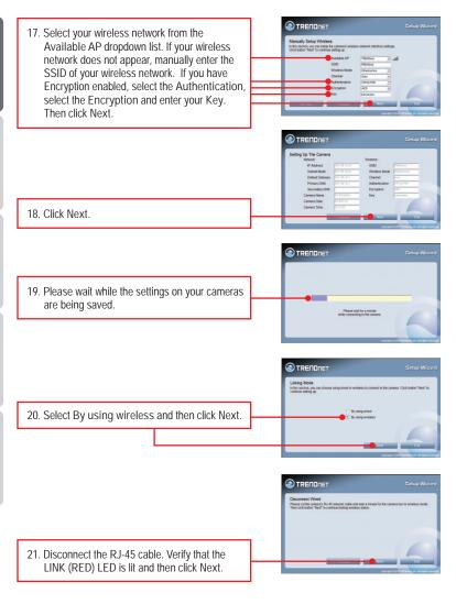
Note: The TV-IP612WN will not work wirelessly until you disconnect the Ethernet cable from the back of the camera.
