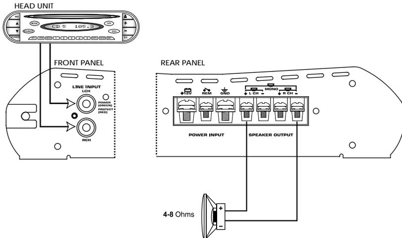
1. Lowest recommended impedance is 4ohm bridged mono
