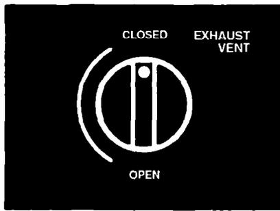
1. Set Exhaust Vent Control to CLOSED for maximum cooling or heating.
