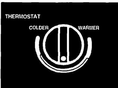
3. Turn the Thermostat Control to desired setting. You can adjust the air conditioner's cooling or heating performance by resetting the Thermostat Control toward COLDER for more cooling. Turn toward WARMER for more heating. You will need to experiment to find the setting which suits you best.
