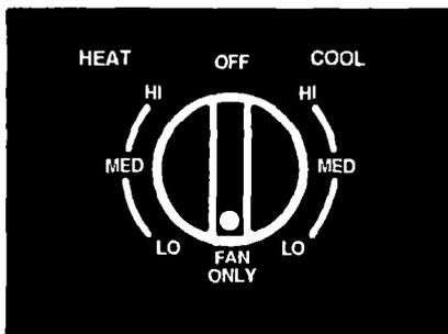
2. Set Fan Speed Control to the desired setting. For cooling, use one of the COOL settings. For heating, use one of the HEAT settings.
