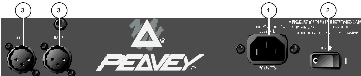
**1. IEC Power Socket:** With the Power Switch (#2) in the off (O) position, plug the power cord into this connector prior to plugging it into your AC power source. **Always insure that proper grounding practices are utilized.** Your SRM uses a universal switching power supply designed to operate with nominal line voltages ranging from 100 to 240 VAC. You may now plug the power cord into the AC power source.
