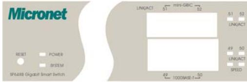
Figure 5. LED indicators of the Switch
