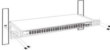
Figure 2. Mount the Switch in the rack
