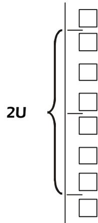
3. Align the mounting holes on the brackets with the caged nuts you installed in step 2, and insert four mounting screws (provided with the rack) to secure the brackets to the enclosure.
