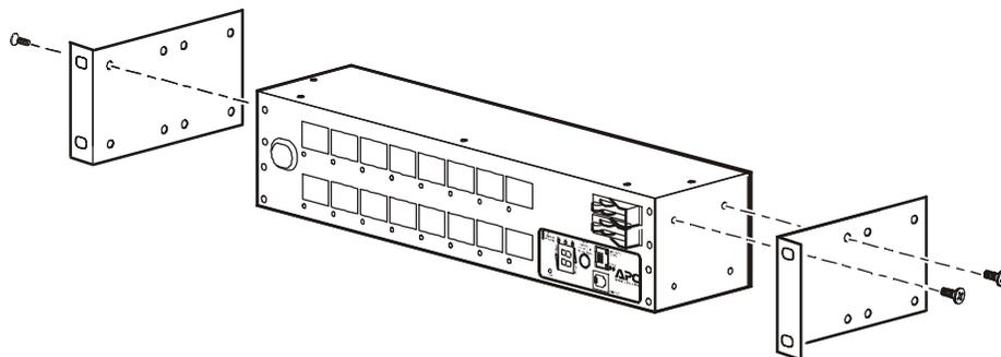
For a recessed placement: use four flat-head screws (provided) through the last four holes of each bracket.
