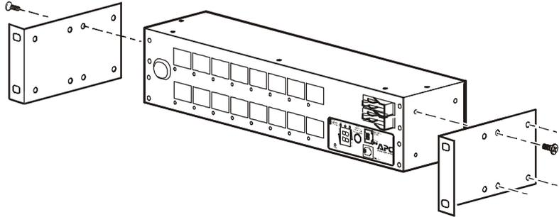
2. Insert caged nuts (provided with the rack) on the vertical mounting rails above a number at the start of two U-spaces in your enclosure and below a number at the lower end of those two U-spaces.
