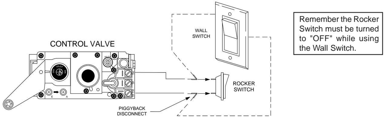
**WIRING WITH THE WTK60 - WALL THERMOSTAT KIT AND THE RCK60 - REMOTE CONTROL KIT:**
