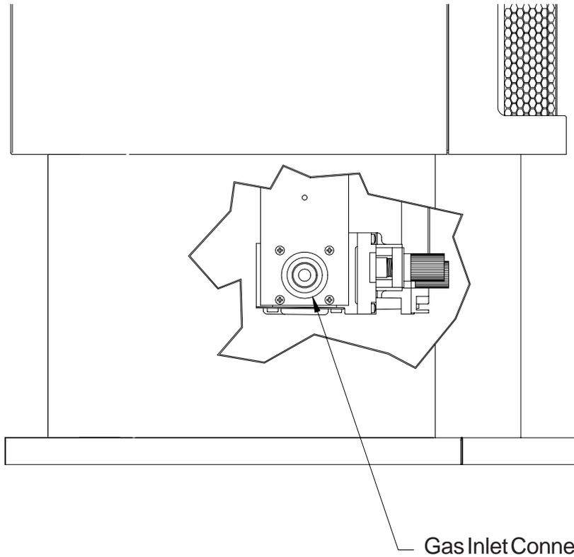
The gas inlet connection is 3/8" NPT, made at the side of the main control through the area at the rear of the pedestal.
