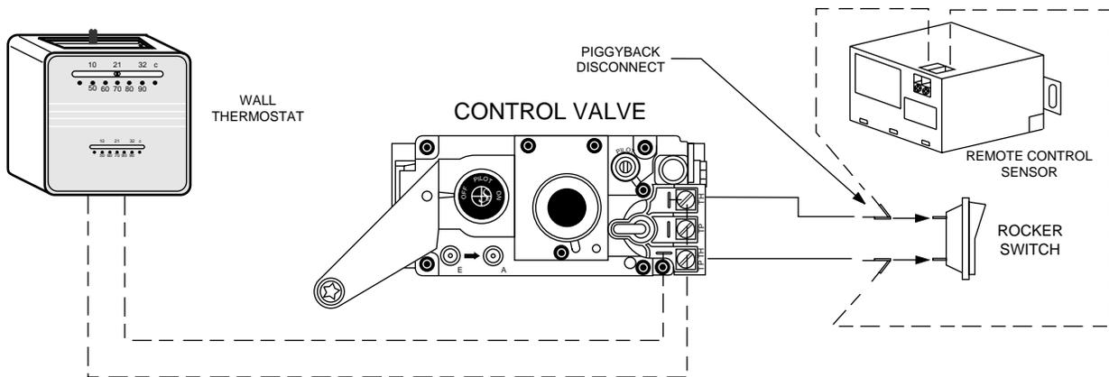
**WIRING WITH THE WSK60 - WALL SWITCH KIT AND THE RCK60 - REMOTE CONTROL KIT:**
