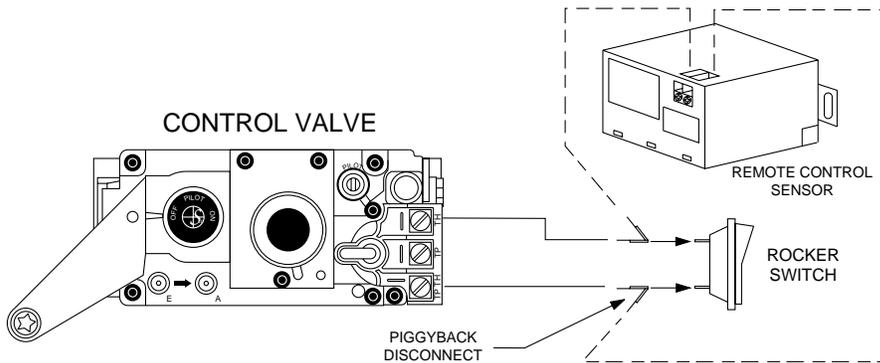
Remember the Rocker Switch must be turned to "OFF" while using the Remote Control.
