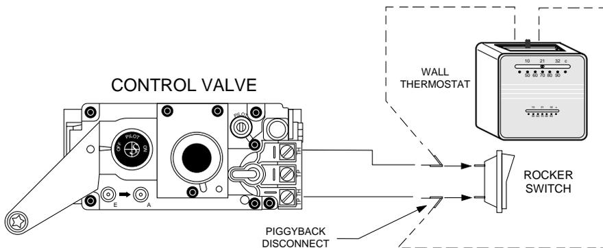
Remember the Rocker Switch must be turned to "OFF" while using the Wall Thermostat.
