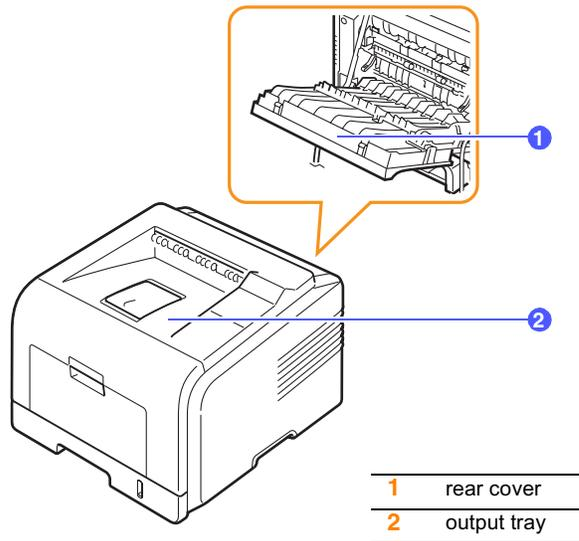
The printer sends output to the output tray by default. To use the output tray, make sure that the rear cover is closed.
