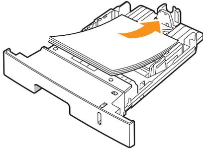
You can load letterhead paper with the design side face down. The top edge of the sheet with the logo should be placed at the front of the tray.
