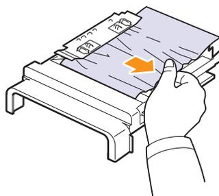
If the paper does not come out with the duplex unit, remove the paper from the bottom of the printer.
