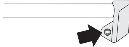
Remove the handrail by removing the 2 end bracket fixing screws.
