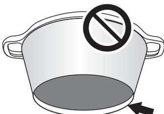
Simmering aids, such as asbestos or mesh mats, are NOT recommended. They will reduce burner performance and could damage the pan supports.
