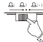
2. Press the **Alarm Set button** to display the alarm 1 time.
