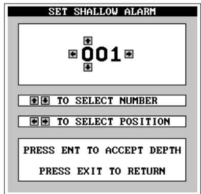
the right arrow key again and press the down arrow key once. This changes the "1" at the end of the number to a "0". The depth now shows 10 feet.
