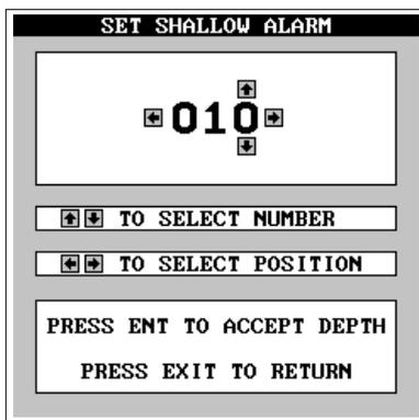
With the shallow alarm set at ten feet, anytime the digital display goes below ten feet, the shallow alarm sounds.
