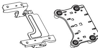
Mount on the back of the computer to adapt the computer for separate wall-mounting hardware (not included).
