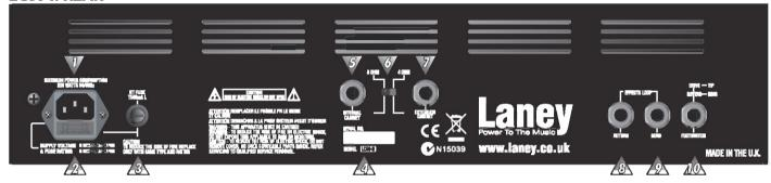
POWER INLET SOCKET. Connect to your power source. Make sure the specified voltage is correct for your country!
