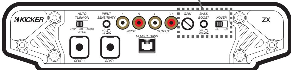
**Automatic Turn-On Selection:** The ZX series offers three different automatic turn-on modes that can be selected on the end panel; +12V, DC Offset, and Audio. Using either the DC Offset or Audio mode causes the REM terminal to have +12V out for turning on additional amplifiers.
