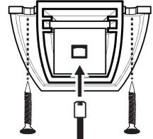
Connect the supplied cable to the KXRC remote and the Remote Bass jack on the amplifier
