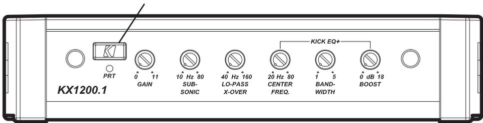
**Automatic Turn-On Selection:** The KX series offers three different automatic turn-on modes that can be selected on the end panel; +12V, DC Offset, and Audio. Using either the DC Offset or Audio mode causes the REM terminal to have +12V out for turning on additional amplifiers.
