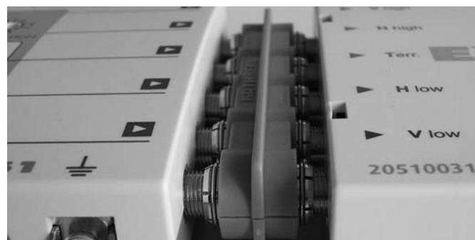
If the units are far apart, it is recommended to use high-quality coaxial cables (with very high screening values) e.g. LCD 111. If possible, use high-quality F-type connectors (see picture right) for "crimping" or compression connectors (see Kathrein catalogue "Satellite and terrestrial antenna products and systems").
