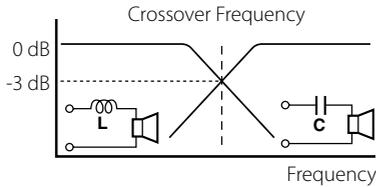
**Coil (L):** Passes low frequencies and blocks high frequencies. (Low pass)
