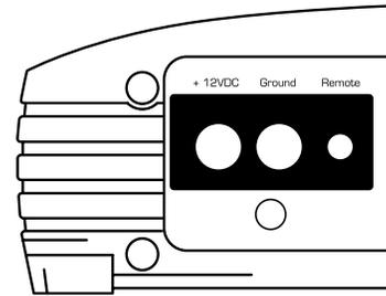
The e1800D's "+12VDC" and "Ground" connections are designed to accept 4 AWG power wire. **4 AWG is a minimum power wire size for this amplifier.**
