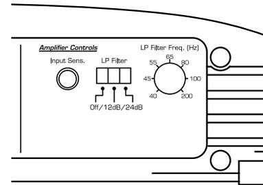
The e1800D employs a sophisticated, variable, low-pass active filter for its internal channel. This feature is designed to attenuate frequencies above its filter frequency, so that the system's subwoofers do not reproduce any audible midrange content.
