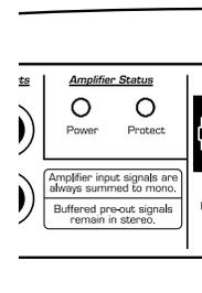
1) "Power" (Green): lights to indicate that the amplifier is turned on and operating normally.
