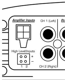
You may run a stereo or a mono signal into the inputs of the amplifier. The amplifier's input section automatically sums stereo signals to mono for the internal amplifier section.
