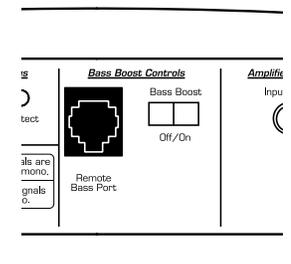
1) **Bass Boost:** This switch allows the user to activate a 6 dB boost centered at 48 Hz. The "Filter Mode" switch in the "Channel 1 & 2" section must be in the "LP" position for the bass boost to be functional.
