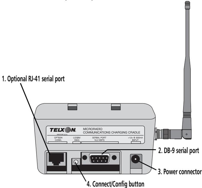
1. This RJ-41 serial port connects the MRC-921 via cable to a host's RS-232 serial port for communication or configuration. Refer to the *MRC-921 Technical Reference* for configuration instructions.
