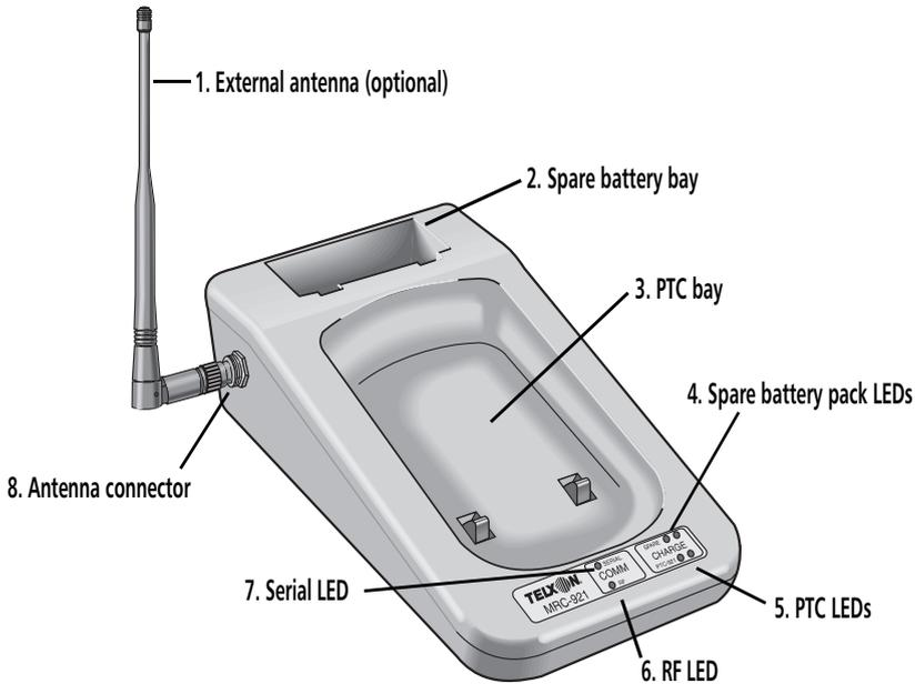
1. An external antenna can be ordered to expand the coverage of the cradle's MicroRadio. Coverage increases from 50 ft (15.2 m) with a standard internal antenna to 100 ft (30.5 m) with an external antenna.
