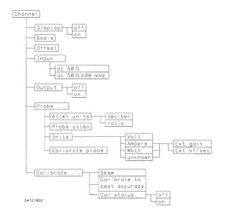
When you press the Channel-Setup hardkey on the plug-in, the softkey menu shown in figure 2 is displayed. This chapter gives you a description of the function of each channel softkey. Some of the softkeys bring up additional menus on the display. A picture of each additional menu is included along with a description of the menu.
