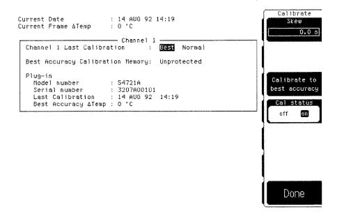
**Current Date** This is the current date and time. You can compare this to the "Last Calibration" time. That way you will know how long it has been since the last best accuracy calibration or normal plug-in calibration was performed.
