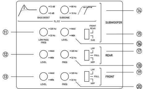
Bass Boost control allows precise shaping of the audio signal for your subwoofer(s). The Subsonic filter is essentially a high-pass crossover which blocks the frequency signal from 10Hz - 80Hz. This signal often contains no music & its removal will improve subwoofer control. The Bass Boost is a variable control to increase the level at 45Hz from 0 - +12dB of gain. Adjust these controls with extreme care.
