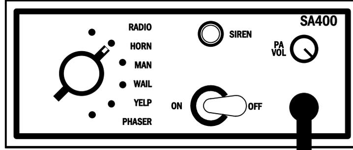
The **OFF/ON** Toggle Power Switch controls the siren power. The siren may be left on any time the vehicle is in operation. The power should be turned off when vehicle is not being used to conserve battery power.
