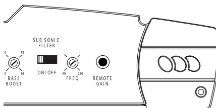
**Note:** If you are using the Remote Gain, make sure to take this into account during set-up procedures of the subwoofer amplifier. You should set the system up with the Remote Gain plugged in, and with the level knob turned all the way down (counter-clockwise).
