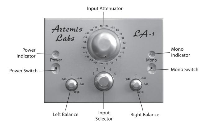
The **Power Switch** applies power when flipped up. The **Power Indicator** will glow red while the tubes warm up, then after approximately 40 seconds, will glow green. About 4 second after that a faint click will be heard, indicating the muting relay turning off. The LA-1 is now ready for use. If the power is removed, even briefly, then restored, the warm-up time delay process will start over again.
