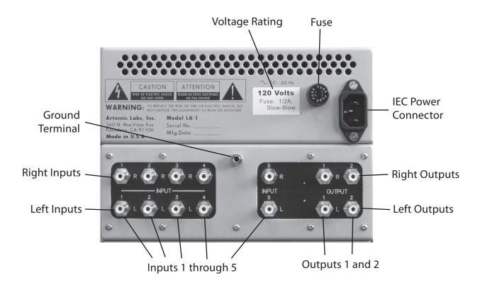
Make sure that the **Voltage Rating** of your LA-1 matches the power mains voltage at your location. The voltage can be changed by internal rewiring, which can be done by Artemis Labs or by a qualified technician. The **Fuse** is a 1" x 1¼" "3AG" Slow-blow type. Its value is given on the **Voltage Rating** sticker.
