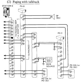
NOTES: (1) One power supply is required for the intercom system and a second power supply is required for the PG-3.
