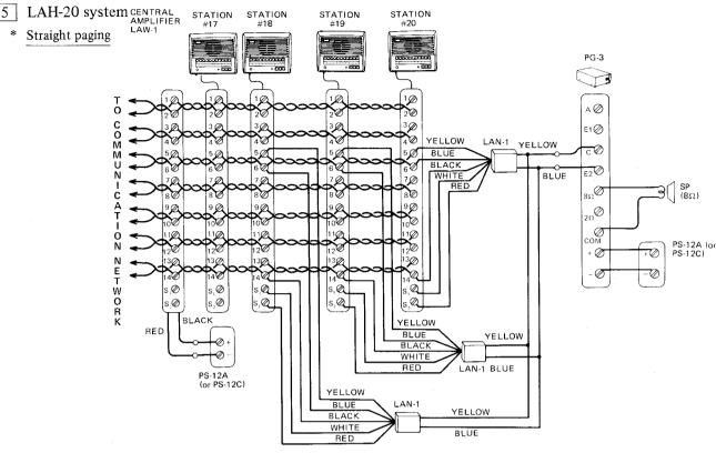
NOTES: (1) One power supply is required for the intercom system and a second power supply is required for the PG-3.
