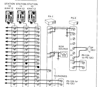
NOTES: (1) One power supply is required for the intercom system and a second power supply is required for the PG-3.
