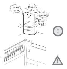
The appliance must be positioned so that the plug is accessible.
