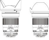
The hood has a bayonet system, which guarantees speedy, efficient, safe and precise installation and will help you take shots that are free of flaring and ghosting. Allign the attachment reference point on the hood with the reference point on the lens. Push the hood onto the lens and turn the hood to the right until it makes a clicking sound.
