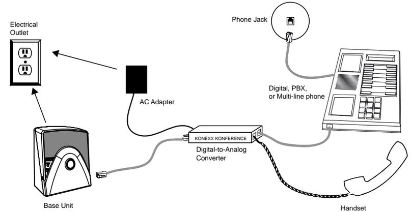
Figure 4. Connecting the base unit to digital-to-analog converter
