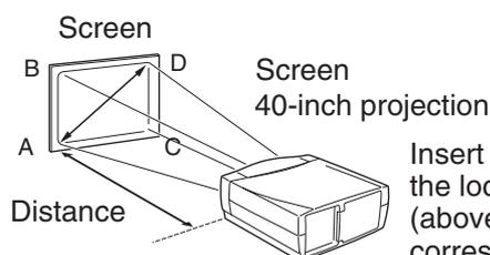
Insert spacers in the location A~D (above figure) corresponding to the screen location A~D.
