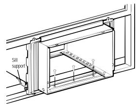
**F** Pull the accordion panels to each window sash track. Attach them on each side to the window sash and the window stool using 4 type C screws.
