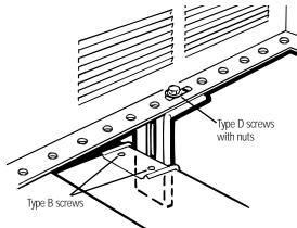
D Adjust the carriage bolts and the lock nuts in each support so that the case is installed with a slight downward tilt (about 1/8"). Tighten the bolts.
