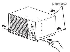
Slide the air conditioner from the case by С gripping the base pan handle and pulling forward while bracing the case.
