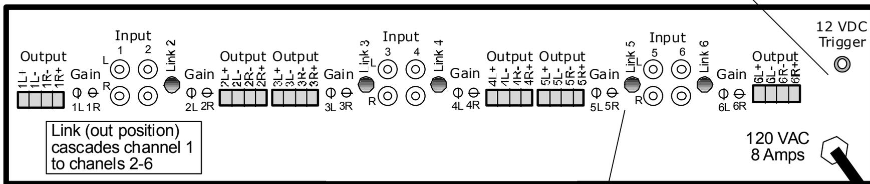
**Caution: NEVER connect the MR1250f to impedances less than 4 ohms or amplifier damage not covered by the warranty may occur.**
