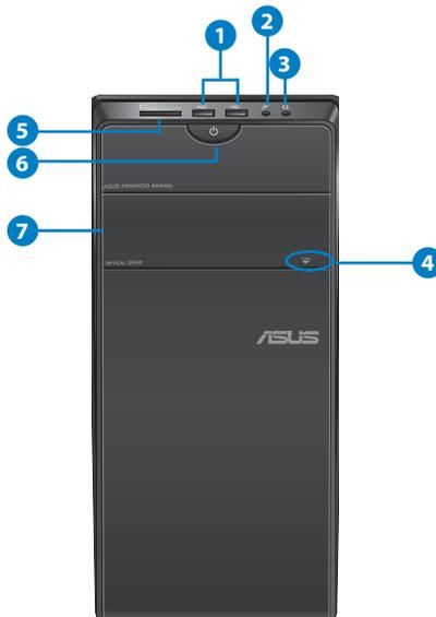
1. **USB 2.0 ports.** These Universal Serial Bus 2.0 (USB 2.0) ports connect to USB 2.0 devices such as a mouse, printer, scanner, camera, PDA, and others.
