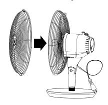
**6** Insert the safety screw into the screw holes and tighten with a Phillips screwdriver.
