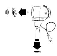
2 Slide the stand into the hole at the center of the base, then tighten the pole locking cap underneath the base.
