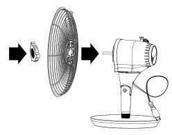
4 Put the fan blade on the motor shaft, then screw the blade cap on to hold it in place. Make sure that the stem of the fan blade is closest to the motor housing
