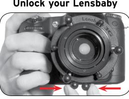
To unlock, squeeze the two Release Knobs at the bottom of the Focusing Collar completely together.
