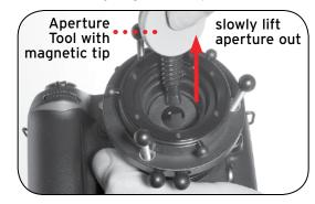
Touch the tip of the Aperture Tool to the Aperture Disk and slowly lift the disk out. Drop in a new disk which is held in place by 3 magnets.
