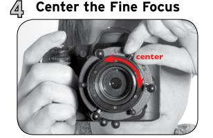
Before focusing, center the Fine Focus Knobs in the middle of their range, midway between the Metal Rods.
