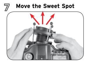
After your subject is in focus, slightly bend your Lensbaby to move the sweet spot of sharp focus. At this point you can take a photograph or lock your Lensbaby. technical support: 1-971-223-5662 While holding your focus, lock your Lensbaby by pressing the button on the top right of the Focusing Collar with your right index or middle finger.
