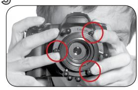
With both thumbs behind the camera place two fingers of your left hand and your right ring finger on the Focusing Collar next to the Fine Focus Knobs.
