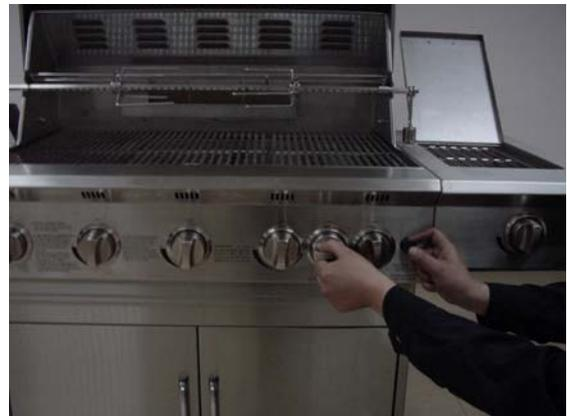
2. Press the electric igniter 3 to 4 seconds to light the rotisserie burner.
