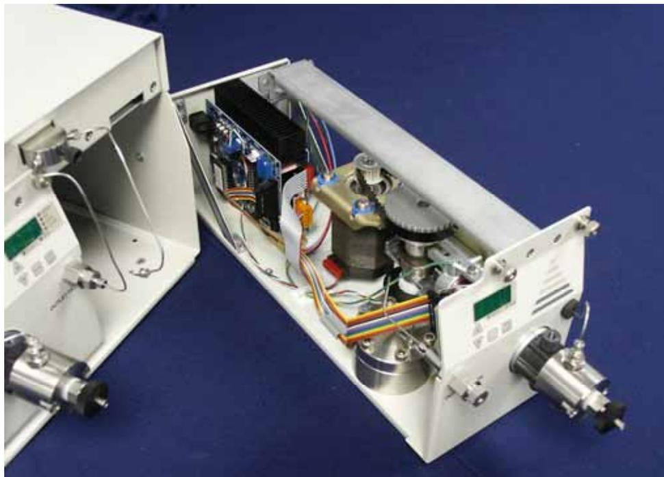
The Pump mechanism, Control Boards, & Pulse Dampener (with Pressure Transducer) are accessible by removing pump drawer.
