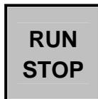
When pressed, this button alternately starts and stops the pump.
