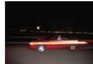
second-curtain sync makes light streaks appear in the path behind the moving subjects, by firing the flash at the end of the exposure
