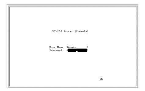
If you're starting the router for the first time, the default login and password is "Admin" – the login and password are case-sensitive, alphanumeric characters.
