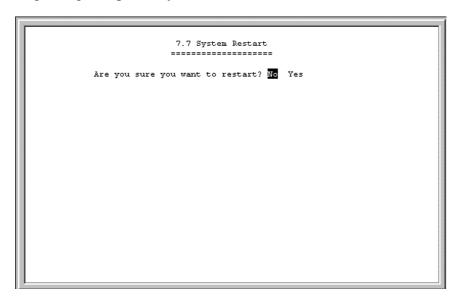
A system restart will not affect the router's settings, but will clear all tables including the routing table and all SNMP counters and tables. It is also used to initiate a software update.
