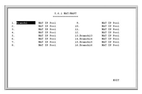
For any NAT entry, you must configure two different screens. The first one is accessible by positioning the cursor over the name field and hitting <Enter> (in the window shown above, this corresponds to the field 'Branch1'). After configuring the NAT options in the Name field, you must save the changes, EXIT, and position the cursor over the NAT IP Pool to configure variables there.
