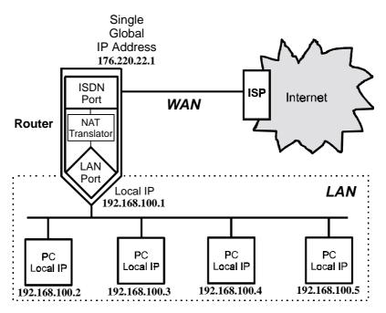
Please note that in the above diagram, the Gateway IP address settings for the local PC's needs to be set to 192.168.100.1, the LAN IP address of the router.
