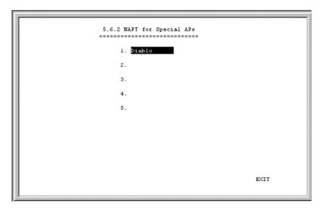
In the above window, position the cursor on any of the numbered name fields and press <Enter>. This will take you to the NAPT configuration screen for special applications shown below.
