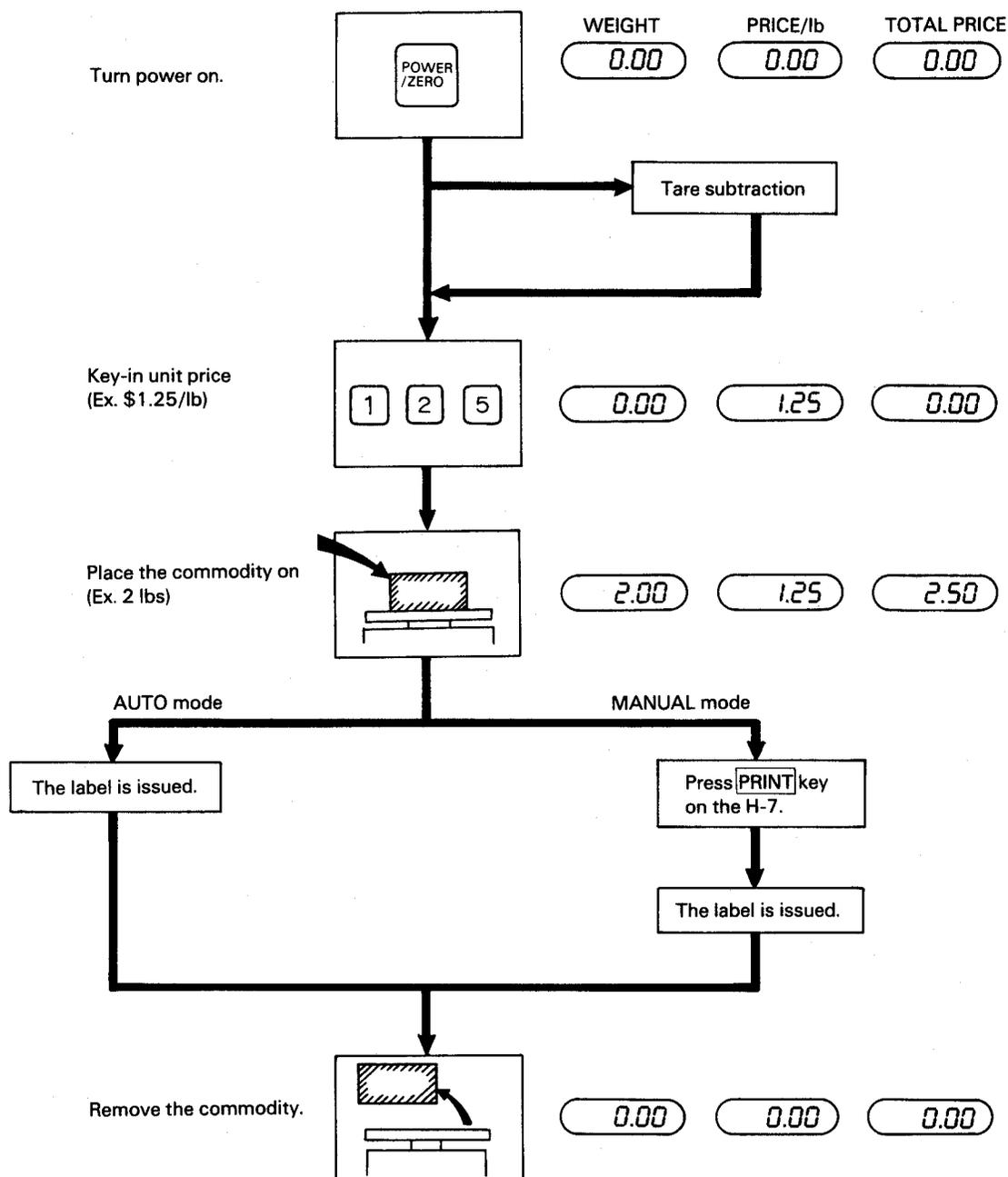
**NOTE:** When the tare weight exceeds 0.20 lbs with the H-7 Label Issue Mode switch set to AUTO position, one tare label sheet will be issued automatically.
