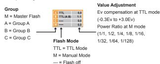
2. Navigate the cursor to **Flash Adjustment** and select the power level ratio between Group A and Group B.
