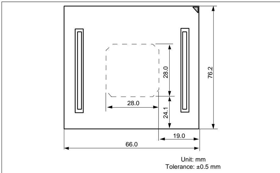
Figure 7 Dimensions for User System Interface Cable Head
