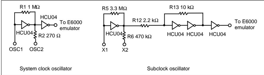
**Figure 10 System Clock Oscillator and Subclock Input Specifications**
