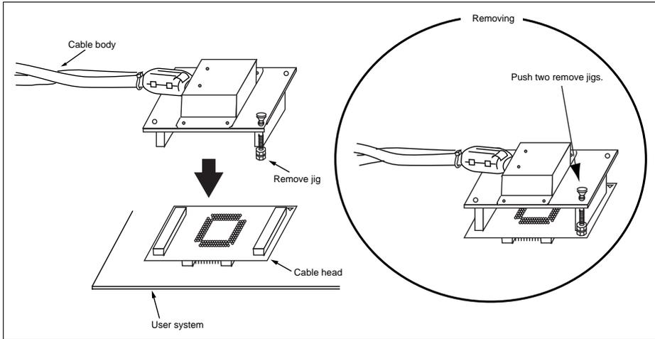
**Figure 5 Fastening Cable Body**
