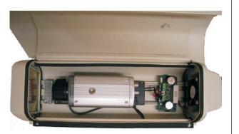
Turn the 1060 housing back to right side up and open the top sideways to allow access to the camera mounting plate fitted to the mounting rails at the bottom of the inside of the housing. Gently prise the base plate up with your hand, or use a screwdriver if this is too difficult.
