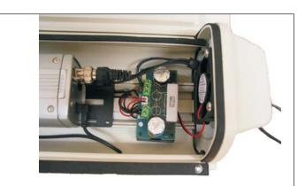
Connect the Video and Power wires you passed through the seal plug to your camera. Connect the opposite end of the cables to a video viewing device and check for correct operation.
