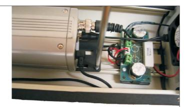
Fit the camera mounting plate back into the mounting rails at the bottom of the housing and push down firmly until it clicks into place. Make any necessary adjustments to the distance from the glass or angle of the camera then screw in the supplied mounting screws to stop the mounting plate from moving.
