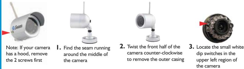
Note: If your camera has a hood, remove the 2 screws first
