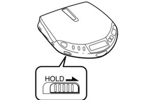
Slide HOLD in the direction of the arrow. The buttons are locked. When you press any button, "Hol d" appears in the display.
