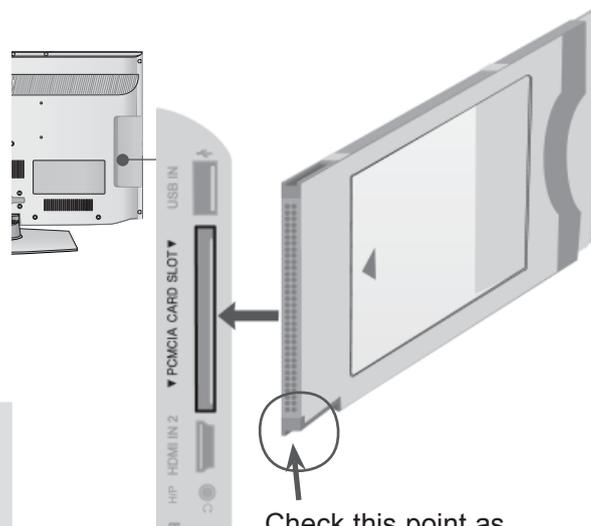
Check this point as shown and insert the CI Module.
