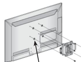
Place the ring spacers on the set before installing the wall mounting bracket so that the inclination of the backside of the set can be adjusted perpendicularly.
