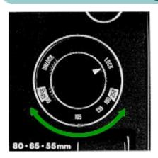
After changing a lens, set the parrallax correcting dial (10) to the focal length value of the mounted lens. For 55mm and 65mm lenses, set the parallax correcting dial to 80, then attach the parallax correction plate for 55mm/65mm lenses to the focusing hood. (Refer to p.22). For the 250mm lens, set the parallax correcting dial to 180.
