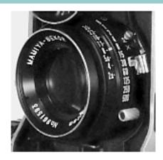
Turn the shutter speed ring and align a desired shutter speed with the index line. The shutter speed ring must be set on a click stop position. Turn the aperture ring and set a desired f/stop to the index line. The aperture ring may be set at intermediate click stop positions.
