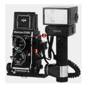
When a falsh unit is used for photographing, connect the synchro cord to the synchro socket (2).
