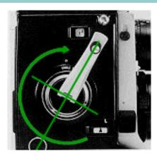
5. Turn the film advance crank clockwise until it stops. The figure 1 appears on the exposure counter at the position where the crank stops diagonally upward, and the shutter is automatically set. Now the camera is ready for the first exposure.
