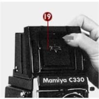
By pushing in the top of the sportsfinder flap (19) at the center of the finder frame, the magnifier swings up into position.
