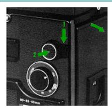
Push the back cover open knob (31) while the back cover lock button (30) is pulled down, and the back cover is open. When the back cover opens, the figure in the exposure counter automatically returns to '0'.
