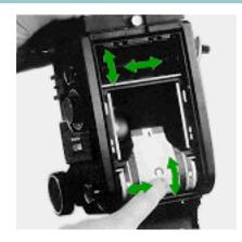
• If either spool change knob is not returned to its original position after loading film, unbalanced film winding will result.
