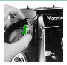
Place the neck strap fastener over the neck strap lug on the camera body and slide it toward the hanging direction while pressing it toward the body until it clicks and locks in place
