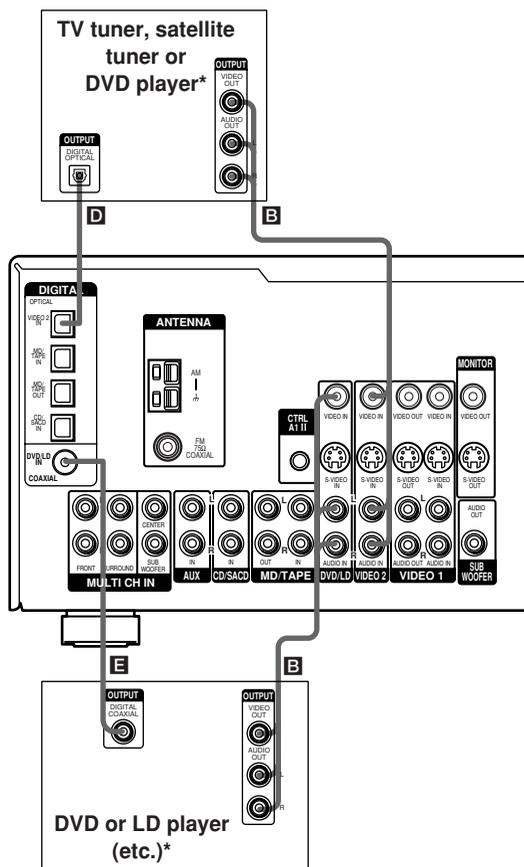
\* Make either coaxial or optical connections. We recommend making coaxial connections instead of optical connections.
