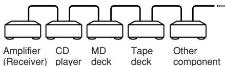
In the CONTROL A1II control system, the control signals flow both ways, so there is no distinction of IN and OUT jacks. If a component has more than one CONTROL A1II jack, you can use either one, or connect different components to each jack.
