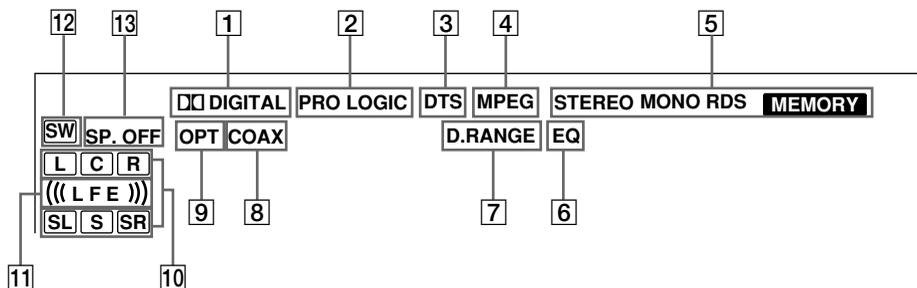
**1** **DIGITAL**: Lights up when the receiver is decoding signals recorded in the Dolby Digital format.
