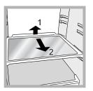
**SHELVES**: with or without grill. Due to the special guides the shelves are removable and the height is adjustable (*see diagram*), allowing easy storage of large containers and food. Height can be adjusted without
