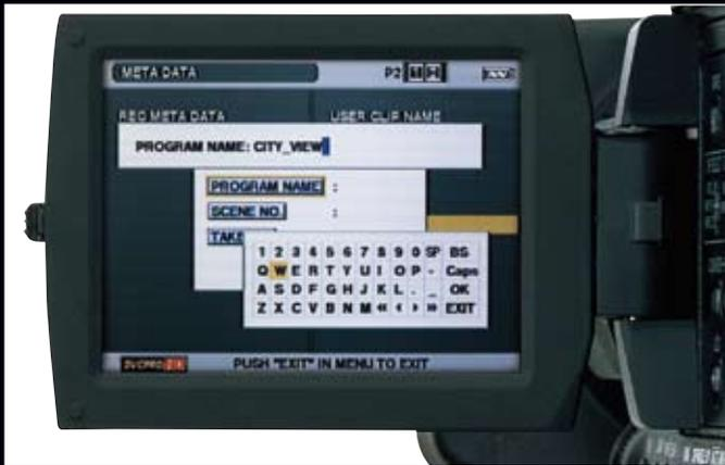
The P2 cam records each recording as a clip (file) and automatically attaches a thumbnail image and file information to it. To preview a clip on the LCD monitor or to check clip data, simply choose the clip you want from the list of thumbnails. It also supports metadata input using a new software keyboard.
