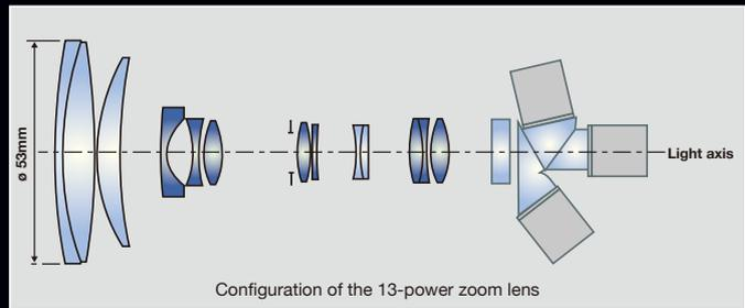
The wide-angle zoom lens that gained high popularity in the HVX200 Series has been reduced in size, lightened, and further widened in this 13x zoom lens. The new lens structure combines 13 lens elements in 10 groups, with 3 aspherical lenses. The diameter of the front lens element has been reduced from 67 to 53.2 mm, while still achieving a 28mm wide angle (35mm equivalent), the widest of the class.\*
