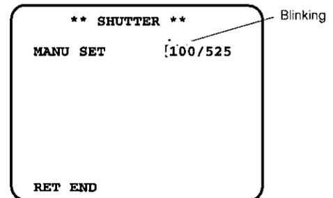
4. Select the desired electronic shutter speed by ◀ or ▶. The adjustable range is 1/525-261/525 lines.
