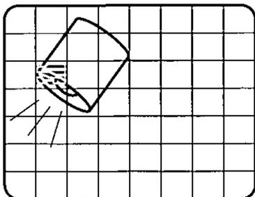
4. Press the PAGE button to mask that area. The mask turns white. (When the cursor is moved on an area that has already been masked, the mask and cursor start blinking.)
