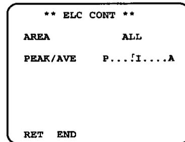
2. Move the "I" cursor to set the detection value. When the "I" cursor is moved to the P (peak) side, the peak value is detected. When the "I" cursor is moved to the A (average) side, the average value is detected.
